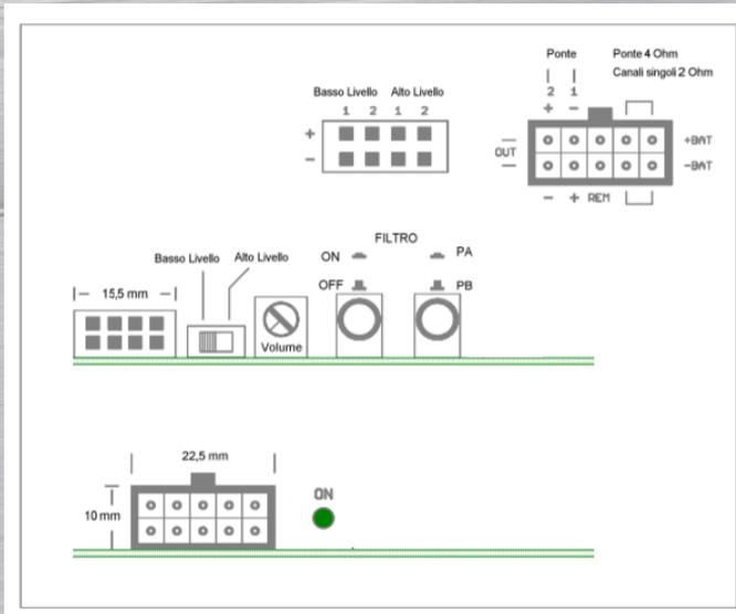
**Status of the amplifier (STATUS).** On the front panel of the amplifier there is the "STATUS" operating status check LED (fig. 1).
